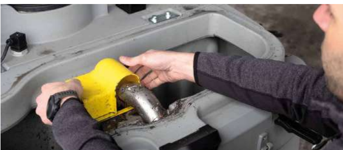
Basket filter to catch any debris, preventing it from settling on the bottom of the recovery tank.
